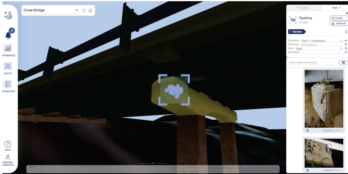
Figure 2: Defects are highlighted on a 3D Model (digital twin) of the asset
